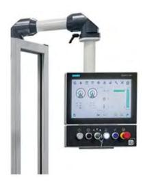
Much of delapena's extensive honing knowledge and best practices are packed into the iHone system, including on-screen help pages enabling the operator to diagnose geometry and finish issues on the machine
