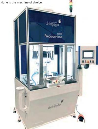
Designed for medium to large batches, the PrecisionHone can be configured to suit the customers' needs. The machine table can be upgraded to a rotary table or x-y table as required. Guarding can be automatic to allow integration of automatic loading systems.
